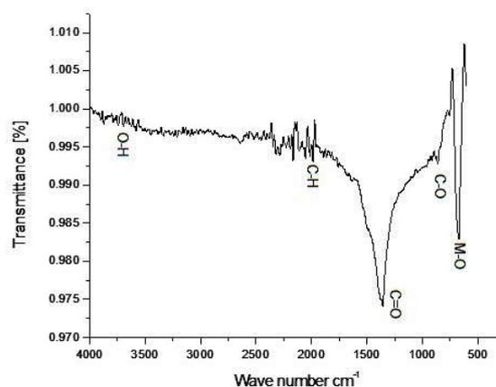
Fig. 1. FTIR spectrum of mixed oxide particles
