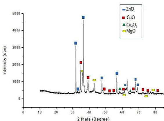
Fig. 2. XRD spectrum of mixed oxide particles
