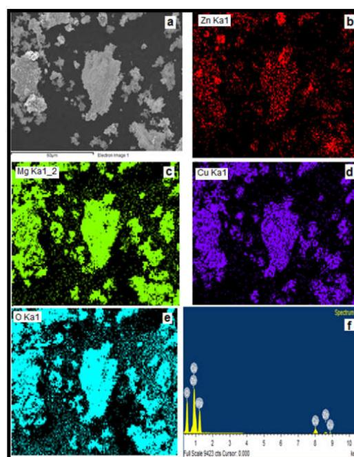
Fig. 3. (a) SEM, (b-e) Elemental mapping and (f) EDX spectrum of mixed oxides
