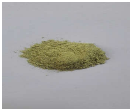
Fig. 1. The \text{Bi}_2\text{O}_3 powder synthesized using Manilkara zapota
