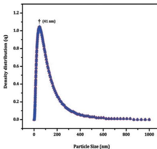
Fig. 7. Particles size distribution of CdS/EDTA nanostructured thin films at 573K
