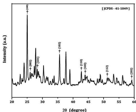
**Fig. 1.** XRD pattern of CdS/EDTA nanostructured thin films at 573 K
