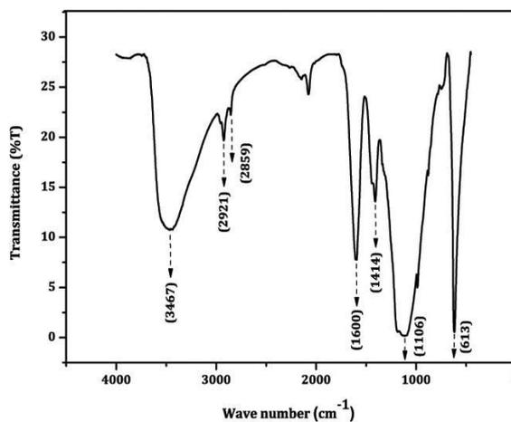
**Fig. 2.** FTIR spectra of CdS/EDTA nanostructured thin films at 573 K
