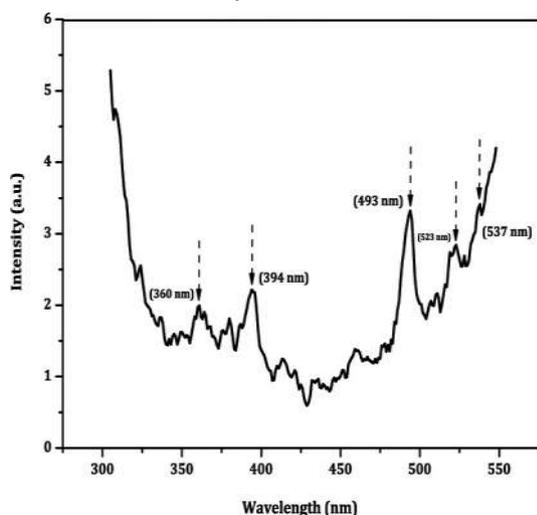
Fig. 5. Photoluminescence spectra of CdS/EDTA nanostructured thin films at 573K
