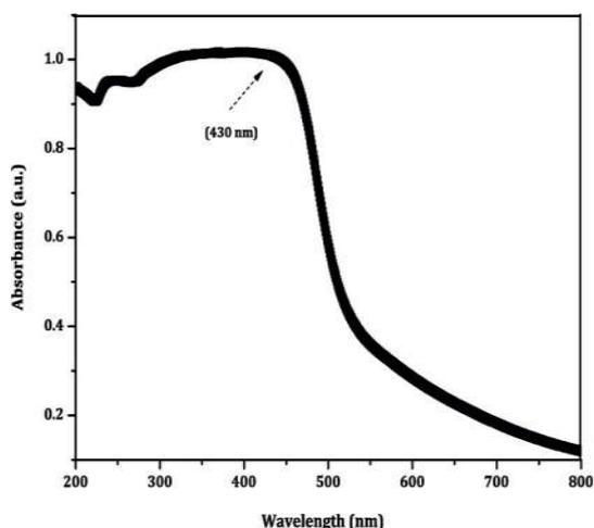
Fig. 4. Optical absorption of CdS/EDTA nanostructured thin films at 573K
