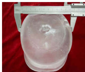
Fig. 1: A photograph of the \text{KCl}_{0.5}\text{Br}_{0.5} single crystal, (\text{KCl})_{0.484}(\text{KBr})_{0.516} in crystal, grown by Li Guo et al. [56]
