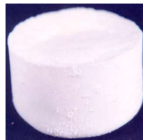
Fig. 3: A photograph of the (\text{NaBr})_{0.1}(\text{KCl})_{0.6}(\text{KBr})_{0.3} polycrystal (multiphased), (\text{NaCl})_{0.068}(\text{NaBr})_{0.032}(\text{KCl})_{0.570}(\text{KBr})_{0.330} in crystal, prepared by Priya and Mahadevan [39]
